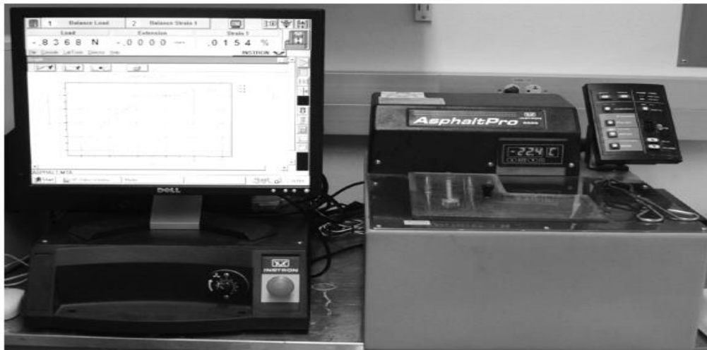
Figure 14 Direct Tension Test Setup
