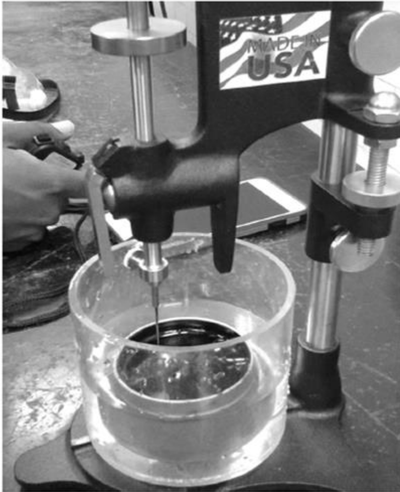
Figure 5 Asphalt Penetration Testing
